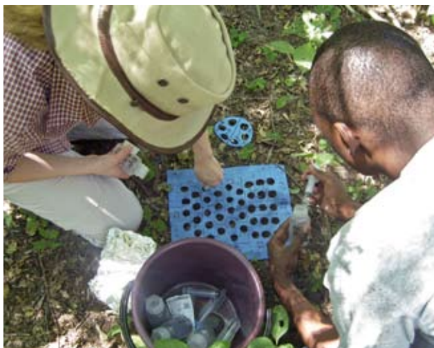
Fig. 13: In situ experiment to determine nitrogen liberating processes i. e. ammonification and nitrification rates under natural conditions (photo: K. Huber).
